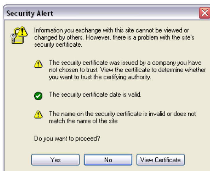
Figure 5.13 – Invalid SSL certificate security alert
