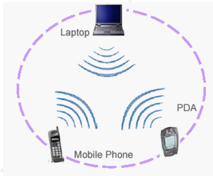
Figure 1. Bluetooth Ad Hoc Topology [6: section 4 page 4]
