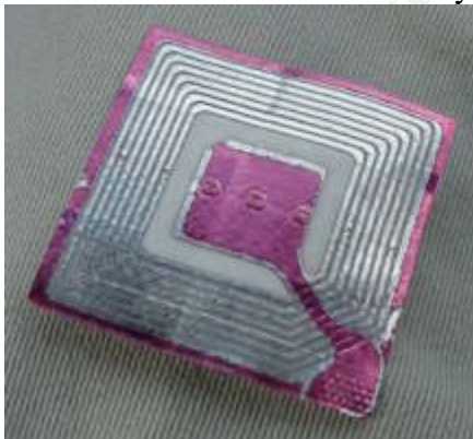
Figure 6: The invisible message side of a Swept RF EAS tag (21). The front likely has a message such as “Thanks for Shopping with us.”
