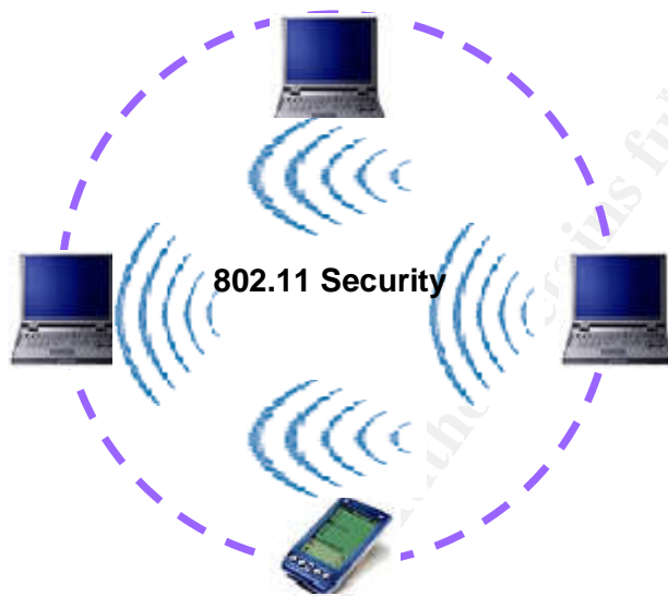
Figure 1 - 802.11 WLAN Implementation In Ad Hoc Topology
