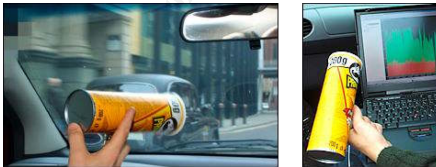
Pringles DIY antenna / receiver 6
