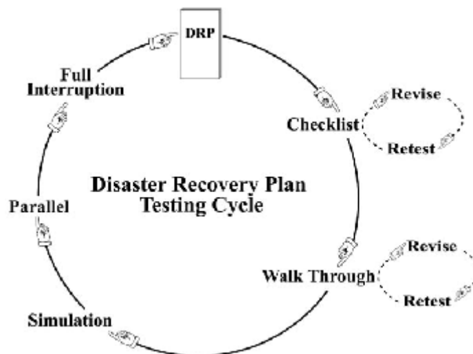
Figure 2. Illustration of a DRP Cycle Testing Scenario
