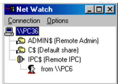
Figure 8 – NetWatch View of remote access using “net use” command
