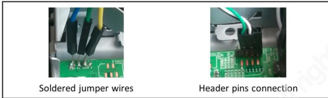
Figure 6. Physical connections to serial port headers
