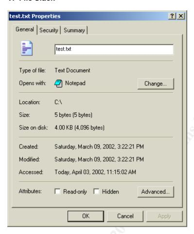
Windows writes files to your hard drive in a minimum of 512-byte chunks to each sector. If you were to open Notepad and create a text file with the word "Hello" in it, it would be 5 bytes in size. As you can see in the graphic above, the file properties report that the file is using 4,096 bytes on the disk.
