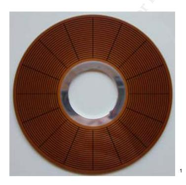
Bytes are stored on some type of magnetic media in blocks of data called sectors. Most computer hard drives and floppy drives use a sector size of 512 bytes. The sector is the smallest unit of storage that computers use to store data. Sectors are created and mapped when the computer storage
