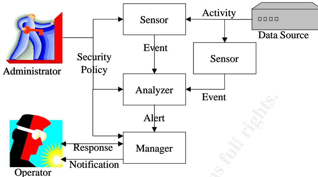
The diagram above illustrates the terms described below and their relationships. Not every IDS will have all of these separate components exactly as shown. Some IDSs will combine these components into a single module; some will have multiple instances of these modules.
