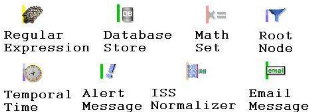
Figure 4: Eight standard operators used in the creation of rules for the correlation engine. Operators manipulate, compare, modify and combine information from the events that are streaming into the SSM product. There are significantly more operators in the full rules set.
