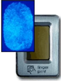
(representative pictures on previous page and left<sup>20</sup>). When the biometric identification devices are built into the laptop proper, without requiring additional external hardware, the biometric scanner hardware and authorization software can be used earlier in the boot up process, denying access more quickly to invalid attempts to boot the system.
