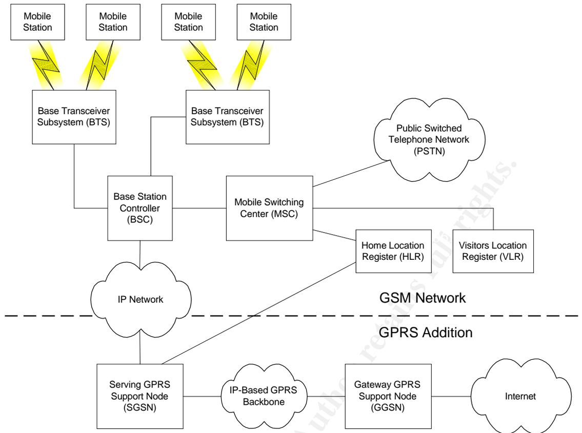
In the above diagram, a Mobile Station represents a wireless device such as a mobile phone. Air Interfaces exist between the Mobile Station and the BTS. Each BTS connects to a BSC. The BSC manages the air traffic by separating voice and data traffic. Circuit-switched voice traffic is directed to the Mobile Switching Center (MSC) and packet-data traffic is directed to the SGSN. The functions of these elements and other GPRS and GSM network components are as follows.
