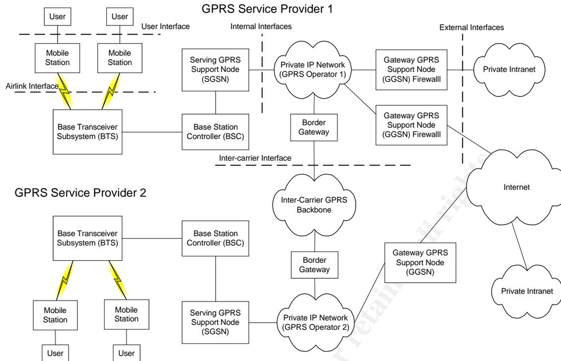
The following is a list of the network interfaces that exist in a GPRS network environment:
