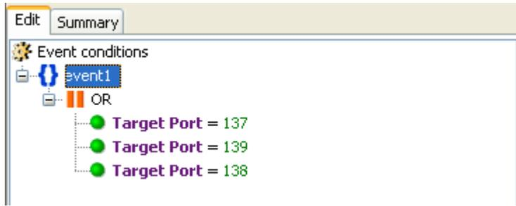
**FIG3 Filter for NetBIOS active channel.**
