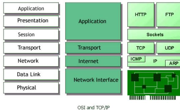
*Figure 2: TCP/IP Model[3]*
