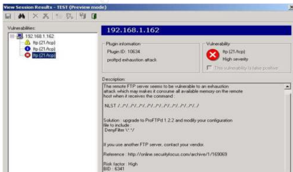
Figure 13 Results from destructive FTP scans.
