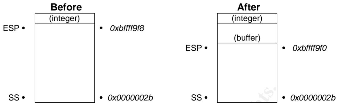
figure 3.2 - Before and after a push operation
