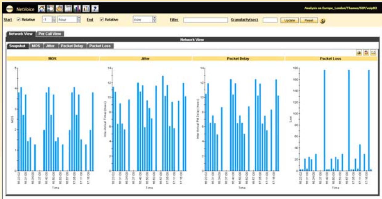
Figure 4: Hourly VoIP traffic load showing MOS, jitter, packet delay and packet loss
