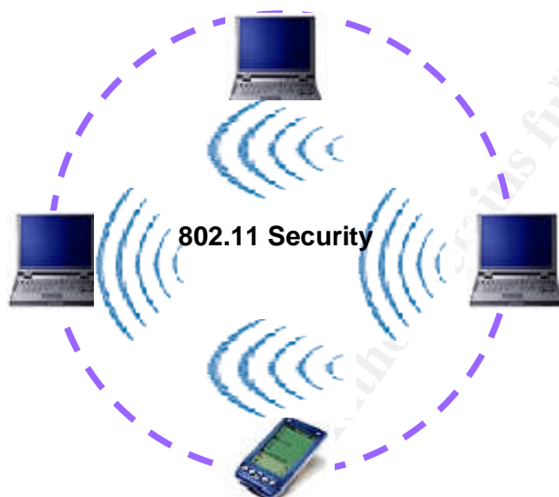
Figure 1 - 802.11 WLAN Implementation In Ad Hoc Topology
