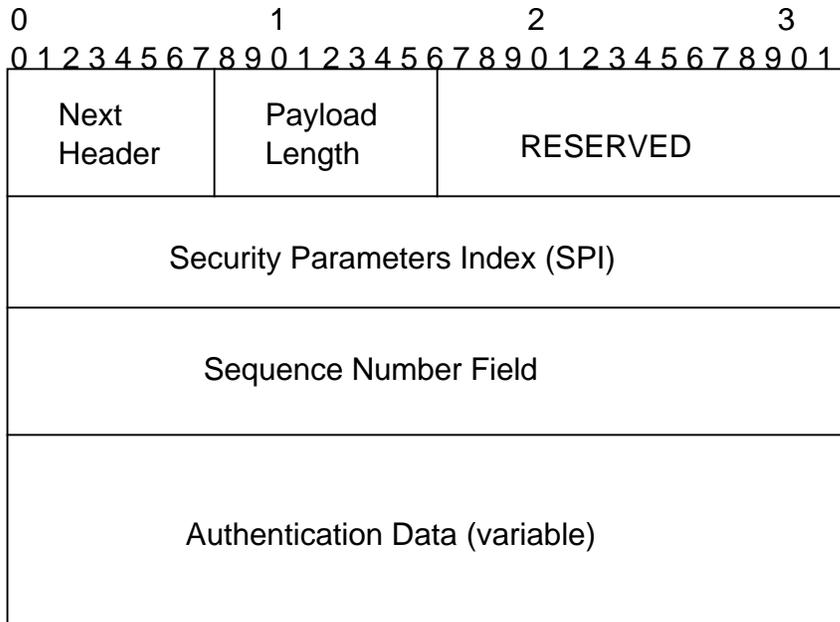
The Authentication Header contains a Next Header field, which identifies the next Extension Header or transport type (e.g. TCP). The Payload Length field contains the length of the Authentication Header. The Security Parameters Index (SPI) field contains the Security Parameters Index to be used in identifying the Security Association.
