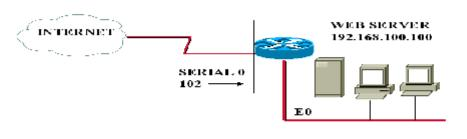
APPLY INBOUND ACCESS LIST TO SERIAL 0. IT IS RECOMMENDED THAT EXTENDED ACCESS LIST ARE PLACED AS CLOSE AS POSSIBLE TO THE SOURCE OF THE TRAFFIC TO BE DENIED
