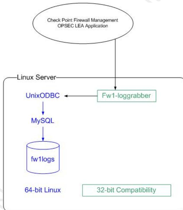
The fw1-loggrabber application on the database server pulls the Check Point log transactions via an SSL connection, then passes the data through UnixODBC to MySQL which stores it in the database.
