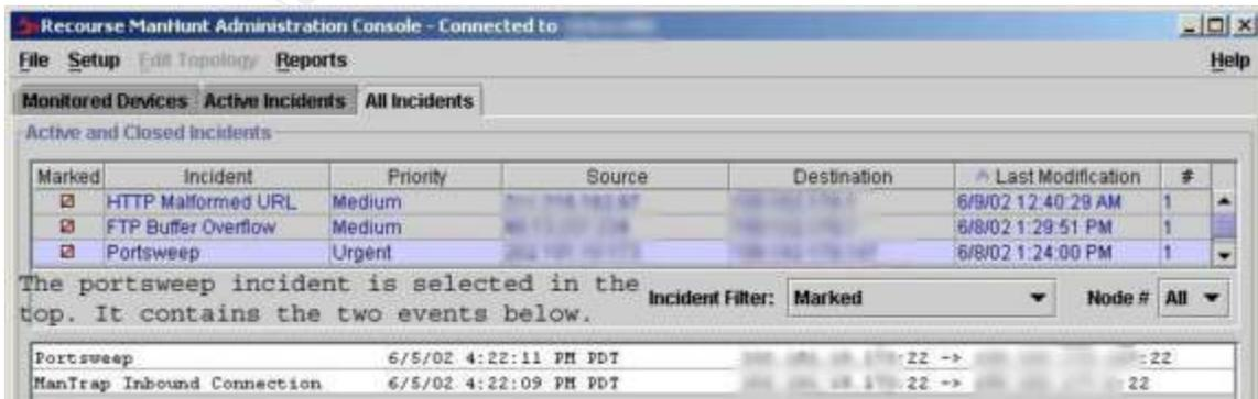
**Figure 2:** An attacker sweeps subnets for open SSH ports. Two sensors detect the probe and the events are correlated as a single incident.
